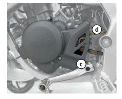
**e)** Now reassemble the cover and the gear lever. When reassembling please make sure to restore the prescribed chain sag of 30 - 35mm. You can easily check this with a folding rule. In addition, you must tighten the rear wheel axle with the intended torque of 7 Nm.
